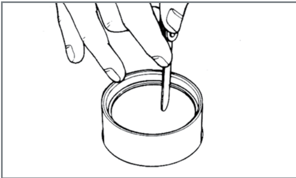
First verification of the piston rings.
