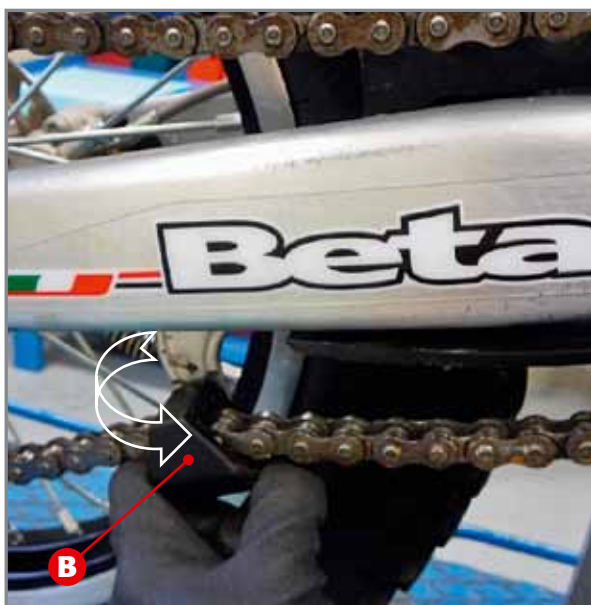
Rotating the chain tensioner
