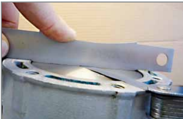
The tool touches the cylinder but don't touches the piston: Measure the clearance between piston and tool.
