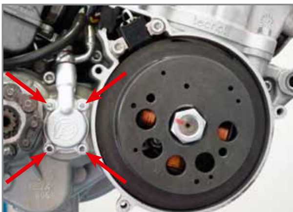
The four screws of the clutch actuator.
