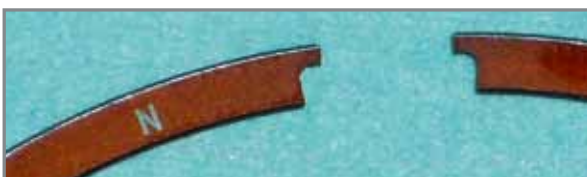
The letter marked on the piston rings.
