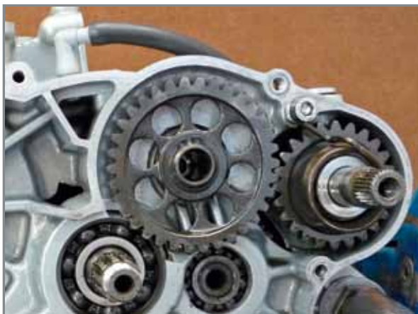
Start-up device assembly coupled with the casing.
