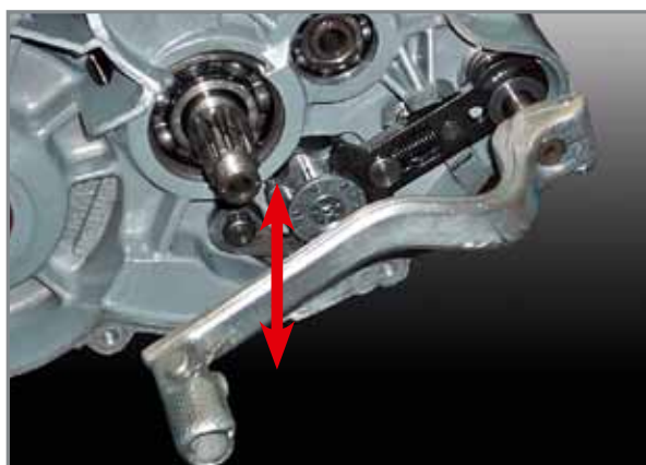
Verifying whether the gearbox unit functions properly.
