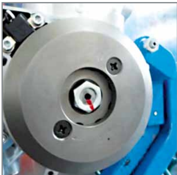
Decoupling the flywheel from the motor shaft by means of extractor B (code 1480210.000)
