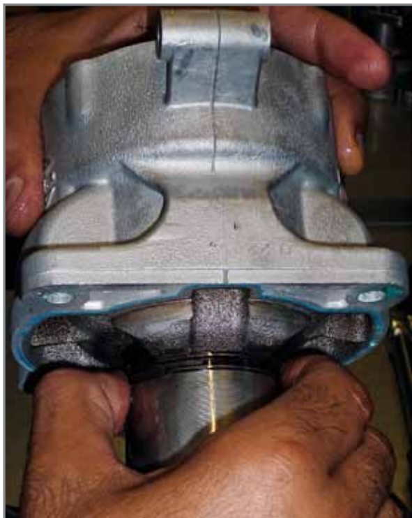
Inserting the piston into the cylinder.
