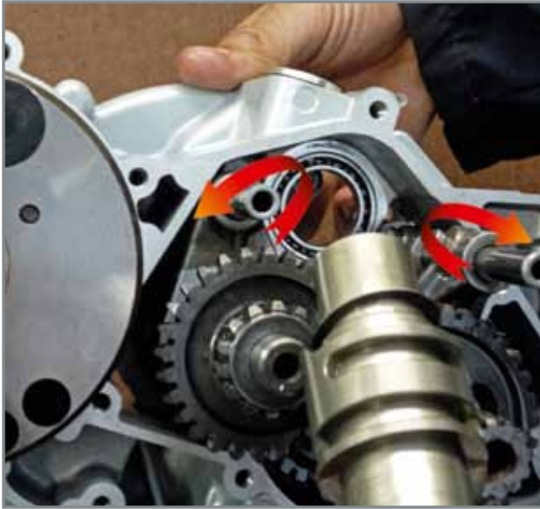
Turning the fork-pin assembly outwards and inserting the desmodromic control device.
