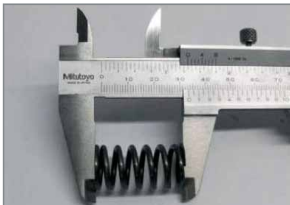
Measuring the length of the clutch springs.
