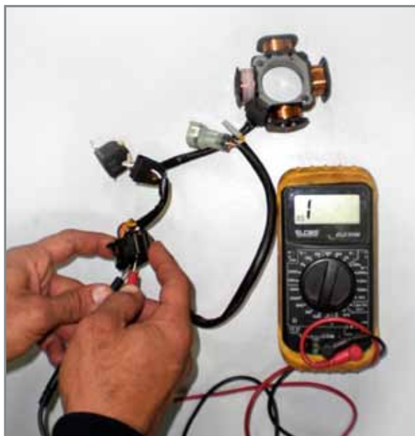
Verifying stator winding functionality.
