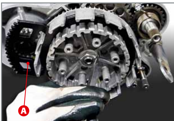
Opening the flaps of the safety washer.
