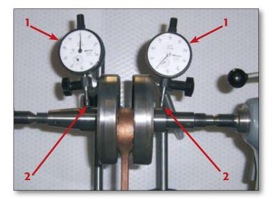
Check for misalignment of the shafts in the crankshaft halves by setting up the crankshaft between centres, or in a similar instrument, and using a pair of dial gauges (1) positioned on the contact surfaces for the main bearings (2) to measure the maximum variation during a complete revolution of the crank.
