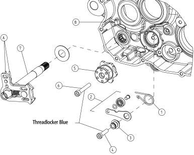
Move the detent lever out of the way and fit the detent cam (5). Secure with the M6x35 bolt (6) tightened to 10 Nm after applying medium-strength thread lock.
