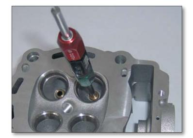
Check the valve stem/valve guide play. To do this, locate the valve in its guide with the top surface of the valve stem flush with the guide, and measure the maximum radial oscillation of the valve head.
