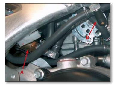
Disconnect the pipes and the electrical connector from the electric tap (A), after making sure that the supplementary/reserve tap (B) is closed (pull the knob downwards).
