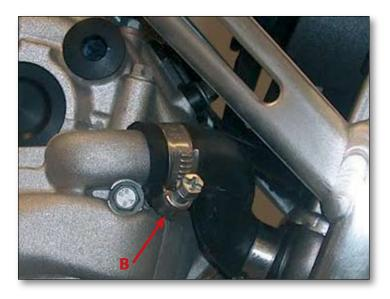
Loosen the clamps that secure the cooling system pipes respectively to the cylinder (A) and the water pump (B).
