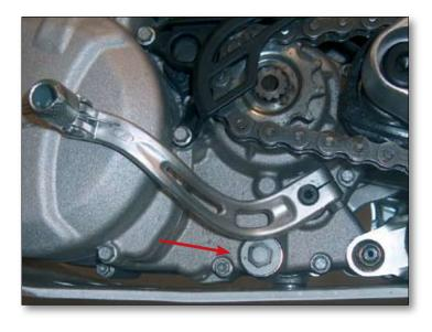
Unscrew the plug in the left-hand casing and use pliers to extract the filter. Clean it carefully and blow it through with compressed air. Check for damage to the O-rings, and replace them if necessary. Refit all the parts and tighten the plug to 15 Nm.
