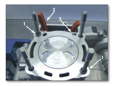
camchain passes freely through the timing case on the right-hand side of the engine.
