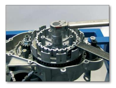
Which locks the retaining nut (9) for the clutch hub (11) and unscrew the nut, using the special tool for locking the clutch centre.
