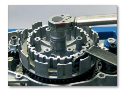
Lock the nut (7) by pulling up the tabs on the tabwasher (A).
