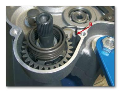
Fit the kickstart idler gear (17) on its shaft, together with the two 18x27x0.5 thrust washers (16, 18), after you have lubricated the parts in contact with each other, and secure it with the circlip (19). Ensure that the convex side of the gear is facing towards the crankcase.
