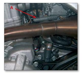
Unhook the tension spring (A) on the side of the exhaust system and the two springs in front of the cylinder head (B).
