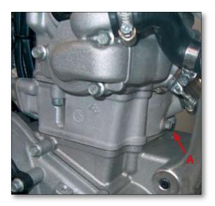
Position a drain pan under the engine and unscrew the drain bolt for the cooling system (A). Then open the radiator cap (B) to allow all the liquid in the system to flow out.
