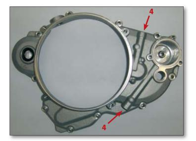
Close the oilways with the special oilway expansion plugs (4), using a pin punch.
