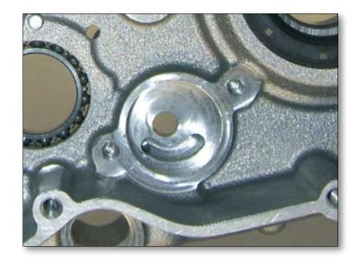
Fit the crankshaft oilseal (12), lubricating its outer surface with grease to make it easier to insert it into its housing. Press it in until it is flush, with the open side facing inwards.
