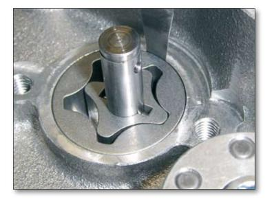
Measure the clearance between the outer rotor and the pump housing, using a feeler gauge for this too.
