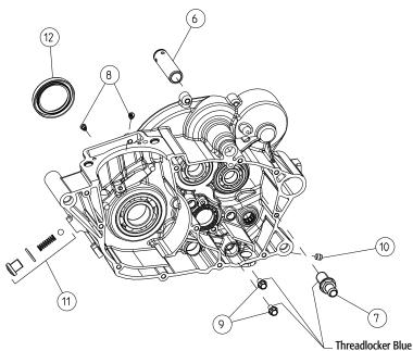
Make sure that the oil pump housing is free from scoring and signs of seizure. Fit the oil pressure relief valve (11).
