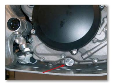
Carry out the same procedure for the output mesh filter, for which the access is via the right-hand engine casing.
