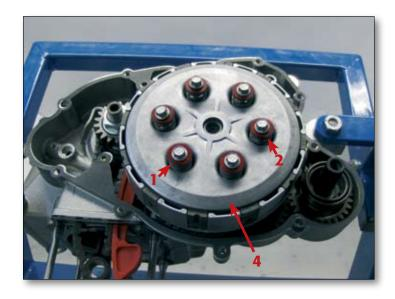
Then extract, in sequence, the special washers (2), the springs (3) and the clutch pressure plate (4). Next, remove the friction plates (8) and then the pressure plate lifter (7), the needle roller bearing (6) and the corresponding washer (5).
