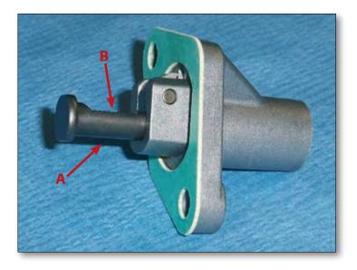
Check that the tensioner plunger (A) moves freely, and check the teeth (B) on the plunger for wear. Before fitting, push the plunger all the way into the tensioner body.
