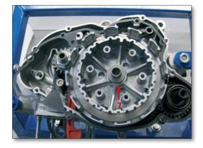
Using a screwdriver, release the tabs on the tabwasher (10).
