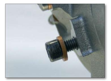
Fit the special washer between the TDC bolt and its housing on the crankcase. As a result, the crankshaft is no longer locked.
