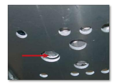
Unscrew the oil drainplug and let all the oil flow out into a drain pan. Thoroughly clean the magnet on the drainplug to get rid of the metallic impurities that it has collected.
