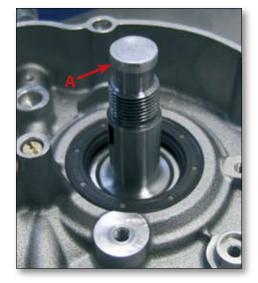
Fit the splitting tool to the right-hand crankcase half, using the threads for the clutch casing bolts to retain it. Then screw in the bolt at the end of the special tool until the crankshaft is extracted.
