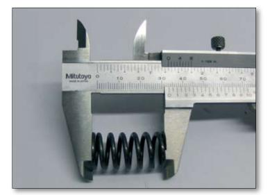
Check the length of the springs (14): Minimum value 33.3mm (33.8mm when new).
