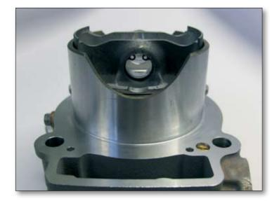
Slide the cylinder down between the studs until the small end of the conrod is aligned with the piston pin housing. Then insert the piston pin from the side which is still open, and lock it with its circlip, having previously lubricated the surfaces of the piston pin itself and of its housing.
