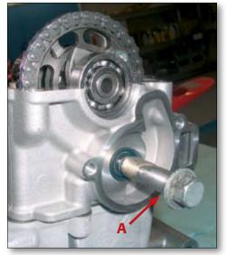
Remove the camchain tensioner by unscrewing the two retaining bolts.
