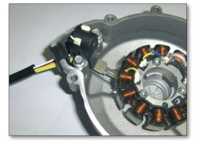
Fit the stator (3) to the flywheel cover (2), retaining it with three M5x25 screws (4). Tighten the screws to 6 Nm. Take care that the stator cable guide plate is facing towards the inside of the cover.
