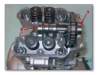
Pass the camchain around the camshaft sprocket, and fit onto the camshaft first the sealed bearing (8) and then the bearing on the chain side (9).
