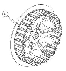
Lock the clutch hub with the special tool and tighten the nut to 90 Nm.
