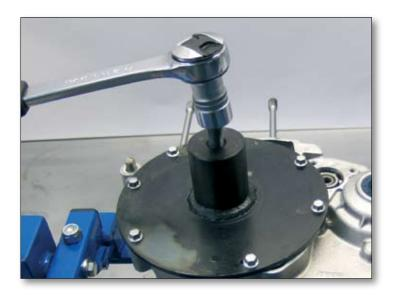
Once you have removed the gasket from the cylinder base, use the special tool for splitting the crankcase, securing it to the left-hand crankcase half using the threads for the flywheel cover retaining bolts. Turn the engine so that the right-hand crankcase half is facing downwards.
