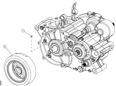
Fit the flywheel (2) and secure it with the flanged nut (3), tightening to a torque of 120 Nm.
