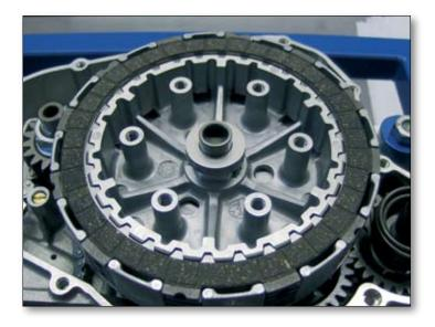
After you have fitted all the friction plates, fit the pressure plate lifter (10) in the central hole in the clutch basket, together with the lifter needle roller bearing (11) and the corresponding washer (12). Check the wear on the needle roller bearing and the contact surfaces. Replace the components if they show excess wear.
