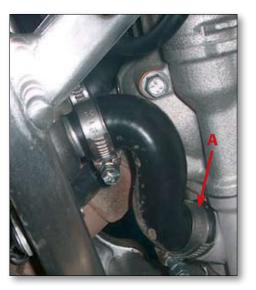
Pull off the sparkplug cap and unscrew the upper bolt (A) securing the coil support.
