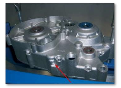
Fit the oilway expansion plug, driving it home with a suitable pin punch.
