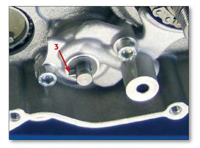
Remove the pin (3) which carries the drive from the gear (2) to the oil pump shaft (8), and then the thrust washer (4). Remove the oil pump cover (7) after first unscrewing the retaining screws (5, 6). Extract the oil pump shaft (8) together with the pin (9), and then remove the oil pump rotors (10), adopting the same procedure as was used for the oil pump in the left-hand crankcase half.
