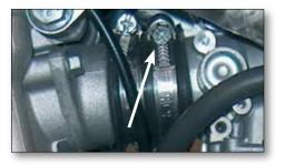
Loosen the clamp (A) which secures the rubber sleeve to the filter box and pull the carburettor backwards (see the arrow in the illustration) until the carburettor is completely disconnected from the rubber flange.
