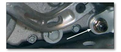
Slack off the nut securing the lower engine/frame mounting bolt.
