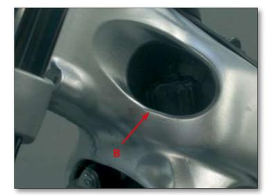
Loosen the clamps that secure the cooling system pipes respectively to the cylinder (A) and the water pump (B).
