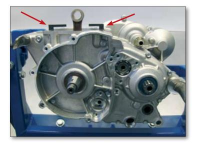
Accurately cut the protruding part of the cylinder base gasket, taking care not to damage the surface on which the cylinder will rest.
