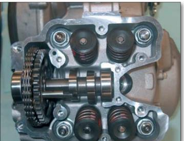
Remove the valve covers and then take out all the bolts securing the cylinder head cover: 2 M6x25 bolts (A), 4 M6x55 bolts (B) and 4 M6x35 bolts (C).
