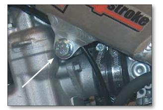
Take out the bolt securing the cylinder head to the frame.
