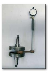
Measure the internal diameter of the conrod small end and then determine the play with the piston pin. If this value exceeds the limit, with the diameter of the piston pin within limits, replace the connecting rod.
