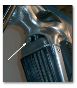
Unscrew the bolt securing the radiator and then remove the entire radiator/stay assembly after disconnecting the connectors for the electric fan and the radiator sensor.
