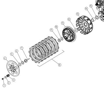
Unscrew the bolts (1) retaining the clutch springs (3) in diagonal sequence to prevent the friction plates (8) from jamming when the springs are released.
