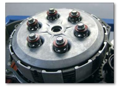
Fit the clutch pressure plate (13), the clutch springs (14), the special washers (15) and the M6x16 bolts (16). Tighten the bolts (16) in diagonal sequence to 10 Nm. Tighten the TDC locking bolt once more.
