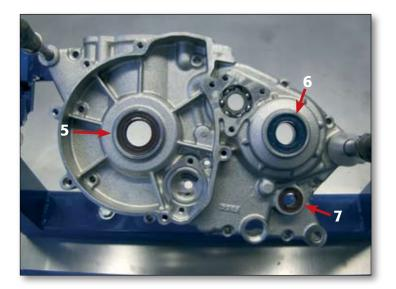
Fit the oilseals for the crankshaft (5), layshaft (6) and gearchange shaft (7), all with the open side facing inwards. Remember to grease the outer surface to facilitate seating.
