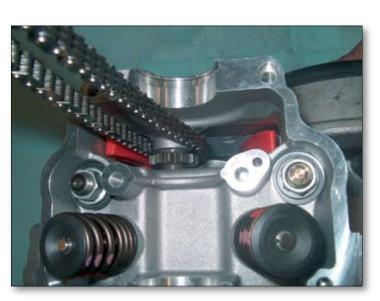
Unscrew the cylinder head retaining nuts, which are screwed onto the studs, and the bolt on the water pump side. Then remove the head and the head gasket, taking care also to remove the dowels.
